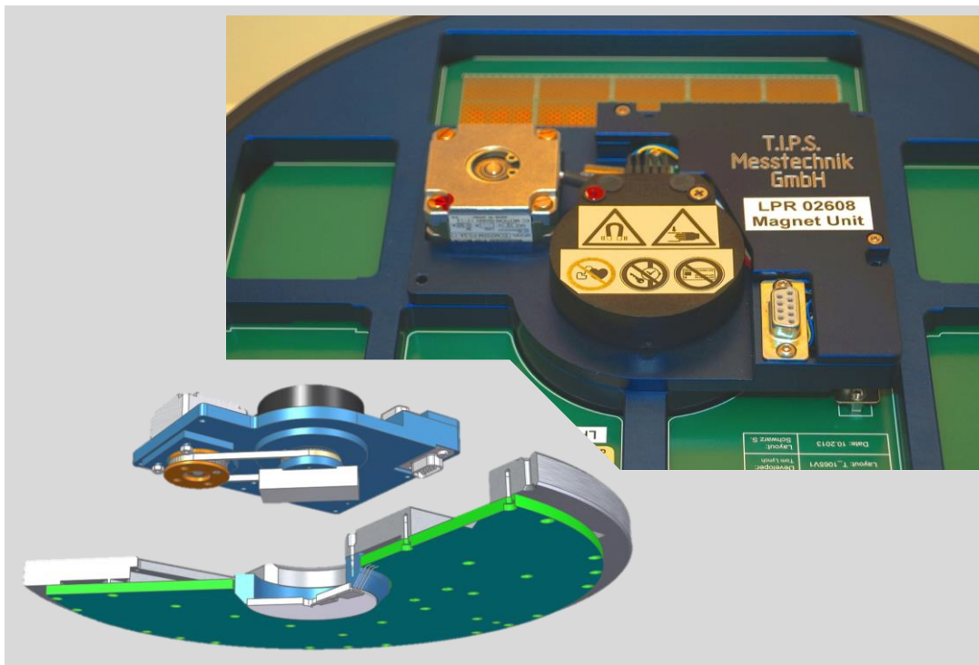
Rotary magnetic unit integrated into Teradyne FLEX probe card: 0.1 ° angular precision, 50 mTesla at device under test
